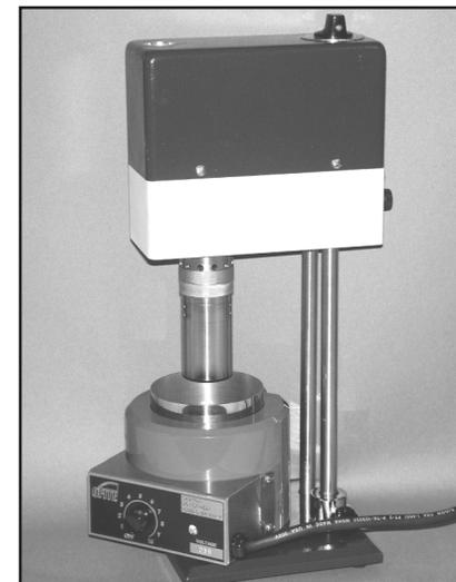
6. Raise or lower instrument to proper depth and stir. Recheck temperature and take reading. Adjustment of temperature may be needed if instrument bob and rotor are cold.
